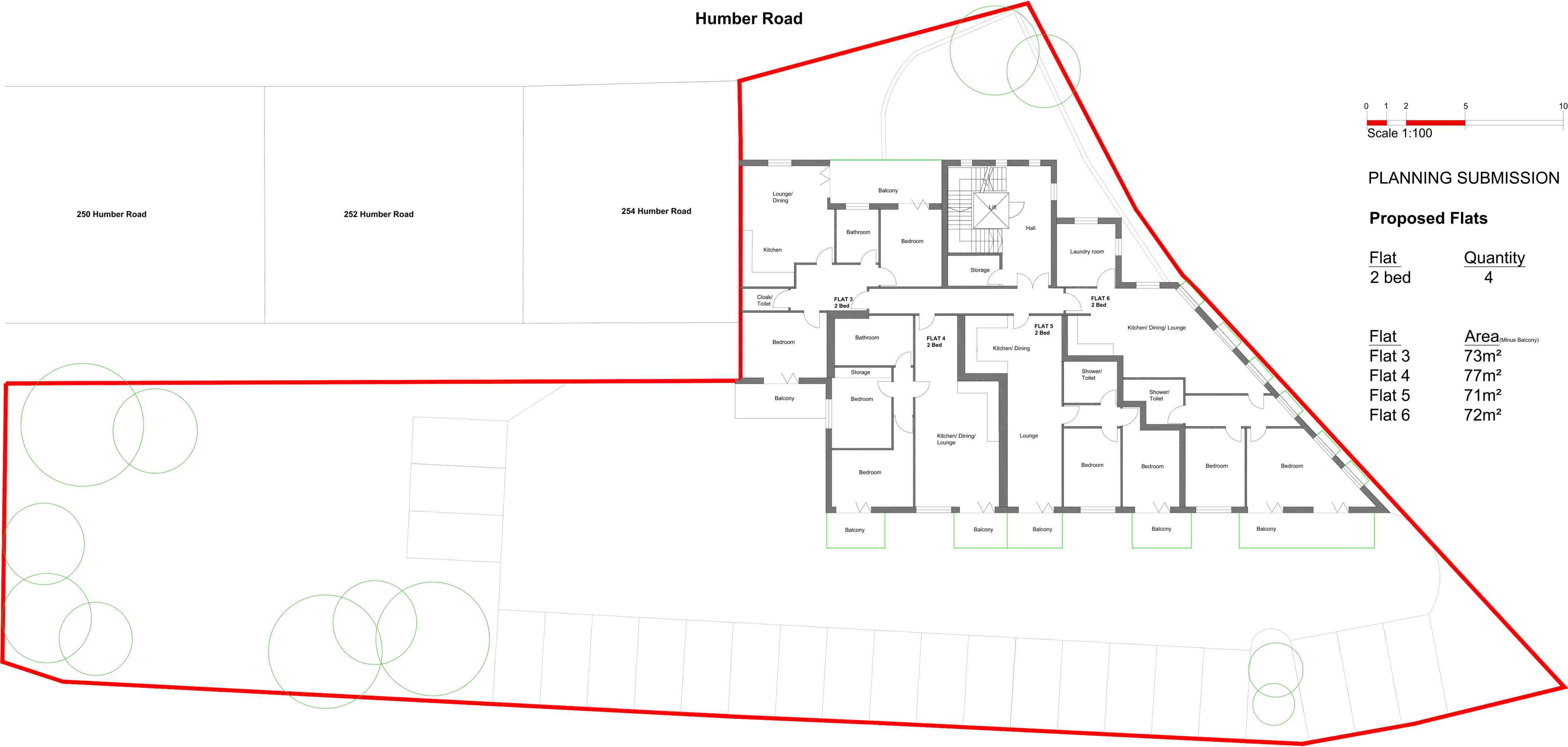
Proposed First Floor Plan Scale 1:100 @ A1
