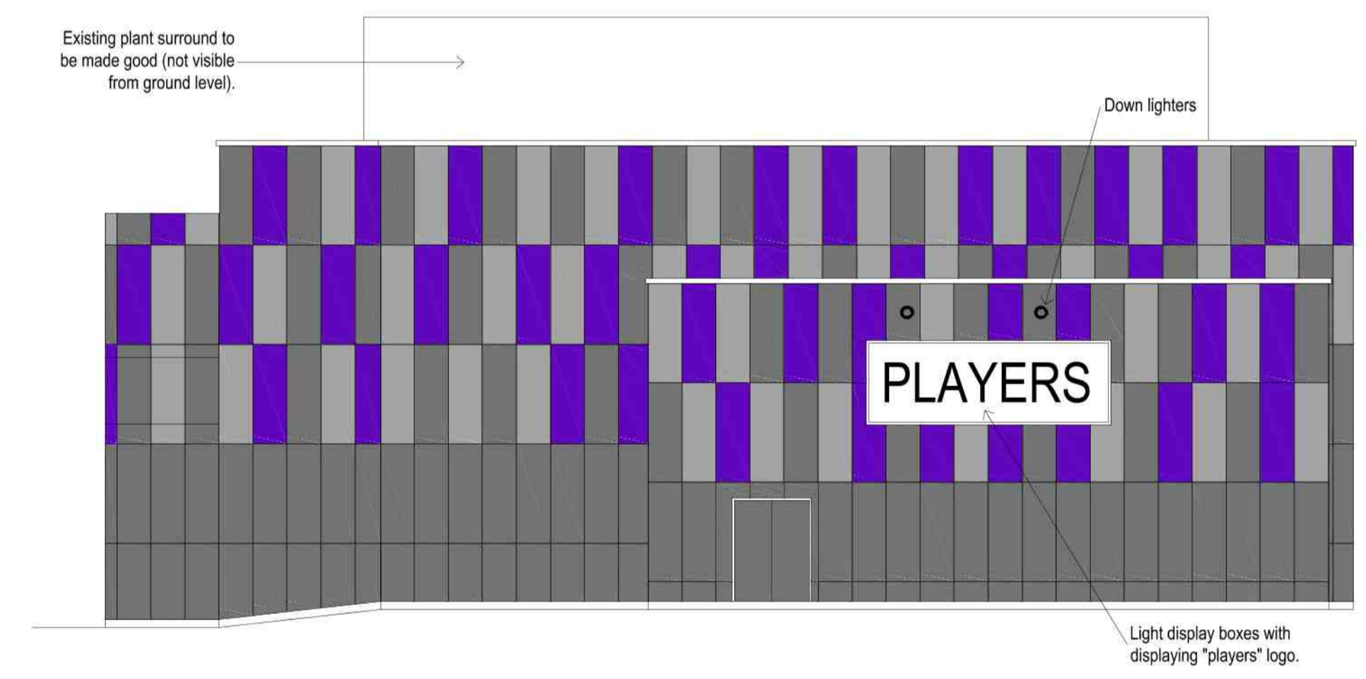
Proposed North facing elevation to Tower Street
