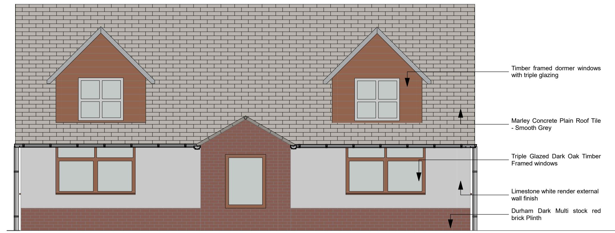
1:50 Front Elevation North Facing HB
