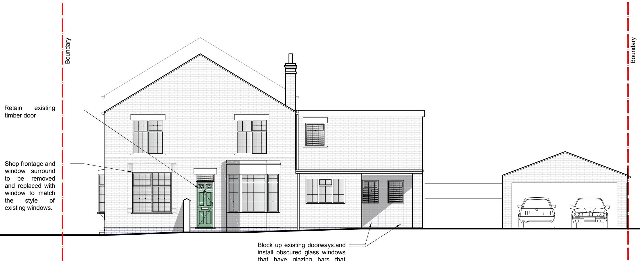
Proposed Side Elevation Abercorn Road 1:100
