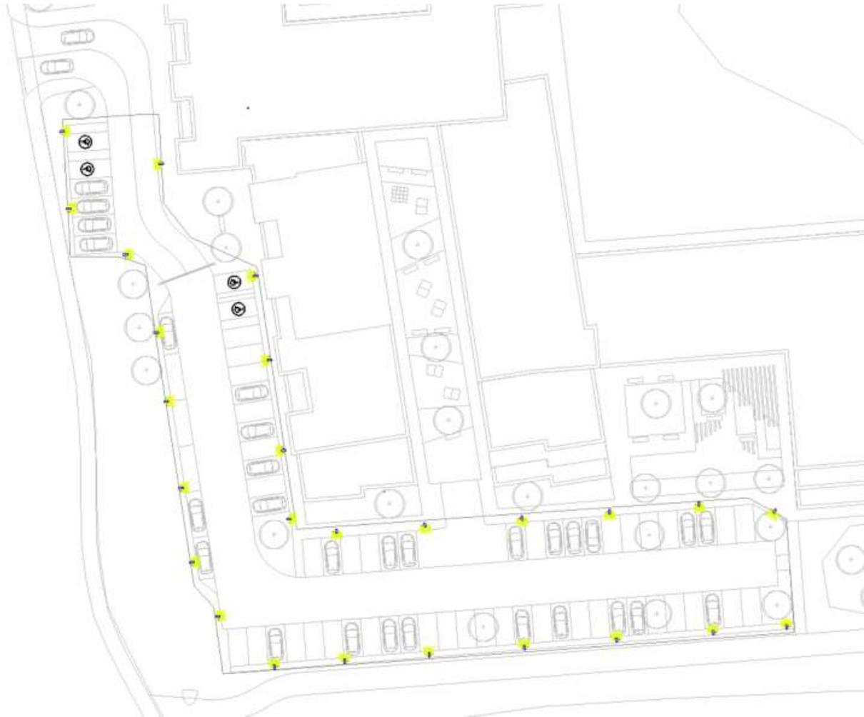
*'Image above indicates proposed location of 4m lighting columns to illuminate the surface car parking area and pathways to the main entrance to the Student Accommodation'*
